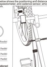
Accessories should be positioned parallel to computer, as shown Computer Function Display Area
