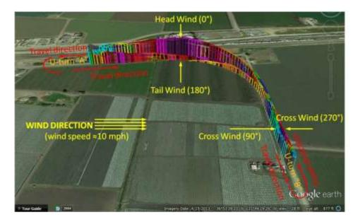
Figure 7 –Wind visualization from data recorded in the iBike power meter using the Newton Tracker app for smart phones. The height of the wall represents "wind speed", a scalar quantity derived from stagnation pressure measured by iBike's wind sensor. The color of the wall represents bike speed.
