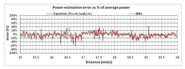
Figure 2 –Error relative to the PowerTap (considered to be the reference), shown over a typical 5 mile section of the same ride. Seemingly random fluctuations in the difference curves appear to be caused by minor timing discrepancies between devices, and diminish with data smoothing. None of the 3 data records stands out as being inherently smoother than the others.
