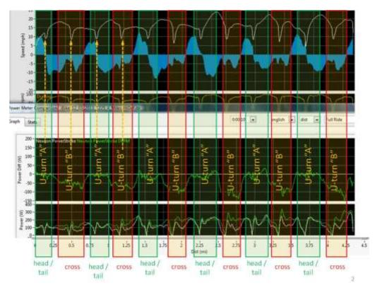
Figure 8 –Data recorded during repeated laps on the course shown in Figure 5. Blue = wind speed. The "Power Diff (W)" plot is the difference between two power meters (iBike Newton and Cyclops PowerTap). In certain crosswind conditions (near U-turn B), the iBike reports approximately 50% less power than the PowerTap. Since PowerTap's accuracy cannot be affected by wind, the discrepancy is attributed to the iBike. Measuring the wind velocity as a vector might have reduced or eliminated this error.
