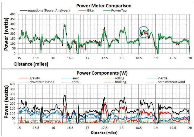
Figure 3 – (a) Typical example of Power Analyzer, iBike and PowerTap power meter outputs. Accuracy in the circled area may be improved with wind angle sensor –see Figures 7 and 8. (b) Total power is divided into 5 constituent load categories. Braking power and the effect of the wind are also shown.
