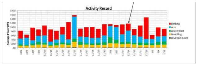
Figure 4 –Activity Chart for an example 10-week period shows each activity's average power (energy also available) and itemizes it in 5 distinct load categories. Note the difference between workouts with similar power levels that are dominated by winds (11/25) as opposed to hills (12/19). The variability of the relative share of acceleration power across multiple activities is also noteworthy (compare, for example, 12/3 with 12/19). Arrow identifies the activity that Figures 1 - 6 refer to.
