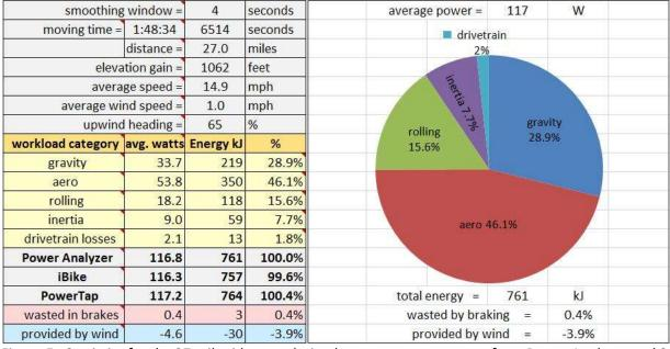
*Figure 5*—*Statistics for the 27 mile ride; correlation between average watts from Power Analyzer and 2 other power meters (iBike and PowerTap).*
