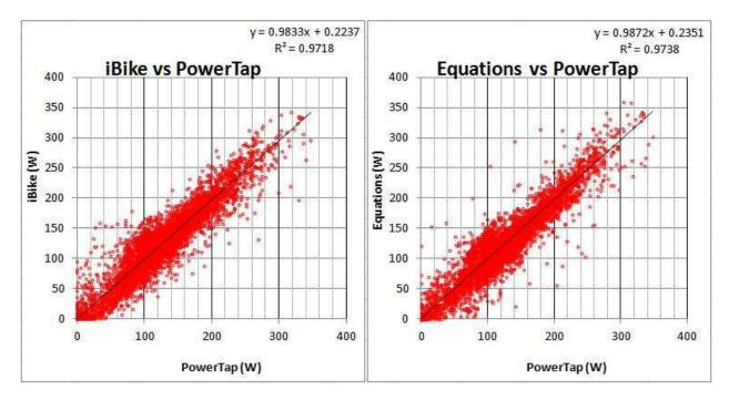
*Figure 1 –Correlation between Equations (Power Analyzer), iBike Newton and Cyclops PowerTap power meters for a 27-mile ride.*
