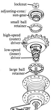
Invert assembly, holding brake arm and hub shell together. Install large ball retainer *ball side down*. Install both drivers as a unit, turning clockwise until seated. Install small ball retainer *ball side down*. Thread on sun gear until it touches planet gears.
