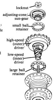
Install large ball retainer ball side down. Install both drivers as a unit, turning clockwise until seated. Install small ball retainer ball side down. Thread on sun gear until it touches planet gears.
