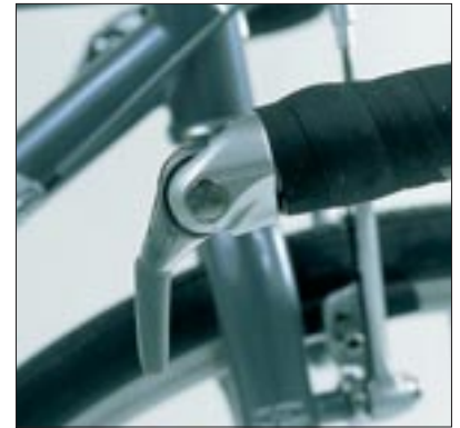
Handlebar-end shifters will work with any front derailleur.
