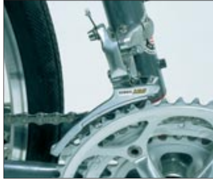
Position the front derailleur cage as close to the chainwheels as possible for good performance.
