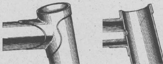
*For all the intriguing parts on the XO-3, the frame, as always, is the heart of the bike. This lightweight frame is built in Japan from thin-gauge butted Ishiwata tubing. Brazed, lugged joints are a clean, stalwart, time-honored method of linking tubes.*
