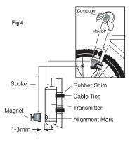
STEP 3: Once the transmitter and wheel magnet are aligned properly, tighten both in place securely.
