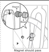
Magnet should pass the center of sensor mark
