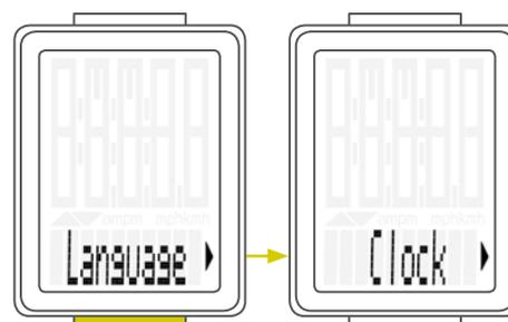
Press the **SET button** to open the setting for the clock.
