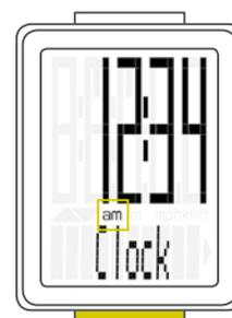
Press the **SET button** to confirm the hour/AM-PM setting.
