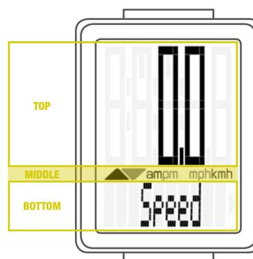
Only **ONE** function at a time appears on the display. To return to the **speed** indicator from a selected function, e.g. **ride time**, press the **SET** button.
