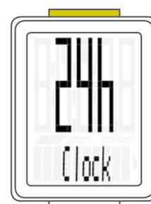
To switch to the 12-hour AM/PM format, press the **BIKE button**.
