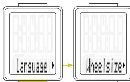
Press the **SET button** to open the setting for the wheel circumference.
