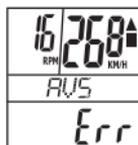
**Note.** If the time or distance is over the max value (29 hr: 59 min: 59 sec or Distance: 999.99km), it will not be able to measure correct average speed by showing "Err" on the displayer. Once the time & distance value has been reset, the average speed will show normally.
