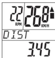
The trip distance accumulated from the beginning onwards.
