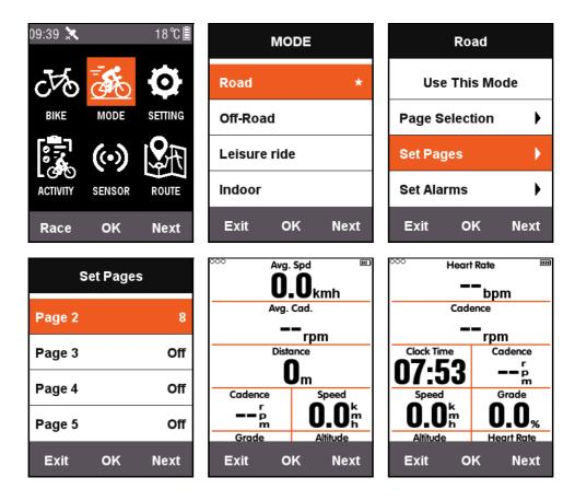
The following is an example to adjust the content displayed on the third field **Distance** to **Clock Time** and describes each step for the display in each field.
