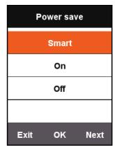
When **Power save** is set to **Smart** or **On**, it will effectively reduce GPS power consumption and increase battery life.
