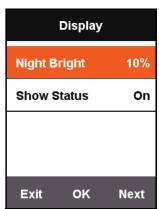
**Show Status** can set up if the satellite signal, activity status and power icon are to be displayed on the top of the screen.
