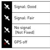
The GPS signal view can display the condition of the current satellite signals received.
