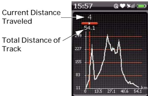
**Figure 23.** The elevation profile
