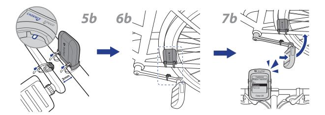
**NOTE:** To ensure optimum performance, the distance between the sensor and the magnet must be within 3 mm.
