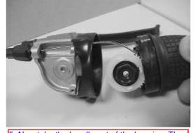
5. Now take the handle out of the housing. The gear with white teeth and handle forms one part.
