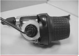
4. Remove screw with Allen key (3 mm).
