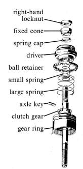
Position axle assembly vertically with right (hollow) end up. Slip gear-ring/clutch-gear assembly over axle with gear ring facing down.
