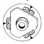
Align planet gears with timing marks facing precisely outwards and install planet carrier (25). Sachs parts list mentions a red timing aid (62) which aligns the gears during installation; correct assembly is, however, possible without using this. Carrier must engage fully over sun gears and turn smoothly. Recheck timing marks after installation.
